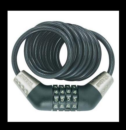
• Cable or coil lock - a many-stranded steel cable enclosed in a plastic casing, with an integrated lock or looped end through which the user secures the shank of an additional lock. The cables come in various thicknesses. These locks are vulnerable to cutting, and thieves can easily sever them using available hand tools.
